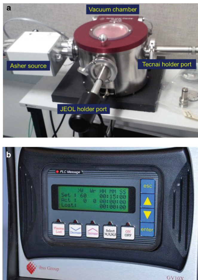
Figure 2: (a) Assembly of the GV10x downstream plasma Gentle Asher system showing the downstream plasma asher source, vacuum chamber, and two TEM holder ports. (b) GV10x controller panel showing the user interface and buttons.
