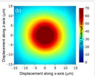
Heat map showing the collection efficiency (in %) of the Lumin SLT parabolic mirror as the STM tip is moved away from the focal point of the parabolic mirror. There is no loss of collection efficiency in the whole scan area even at room temperature.
