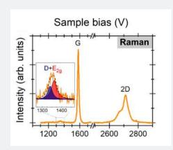
Raman spectrum of HOPG with a single layer (monolayer) of h-BN measured without the STM tip near the sample surface. The spectrum was acquired using a 532 nm laser. ‡
