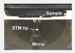
Orientation of the STM tip, sample and parabolic mirror viewed along the optical path from outside of the UHV chamber. Multiple CCD cameras with the mirror's encoded nano-positioners, provide a safe probe approach protocol.
