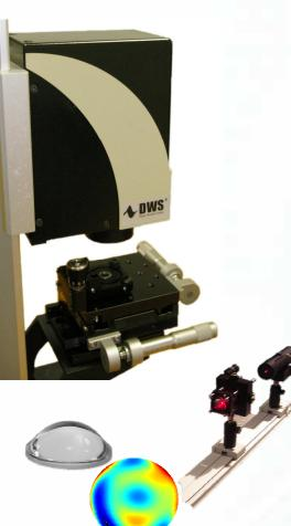
Based on the latest advances in wavefront analysis **WaveGauge**<sup>®</sup> is the ideal wavefront sensor for optics and microlenses quality control or laser beam analysis.
