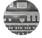
SEM image Logic Device – 65 nm technology. Source: FEI Company
