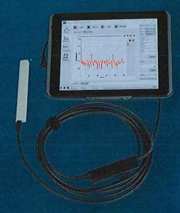
**THM1176 and TFM1186** magnetometers: ultra-compact and easy-to-use instruments to measure and map all three components of a magnetic field using Hall and Fluxgate technologies.
