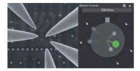
From the main window, the operator is guided through the steps of setting up his nanoprobing system and test recipes, landing probe tips on the device under test, acquiring measurement data and reporting about them.
