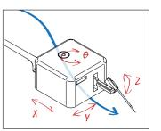
The different operating modes of the piezo actuators provide up to centimeters of travel range with scalable positioning resolution from micrometers to nanometers. The coarse positioning mode saves time when approaching the region of interest, while the fine positioning mode allows for a precise contact landing of the probes at the destination.
