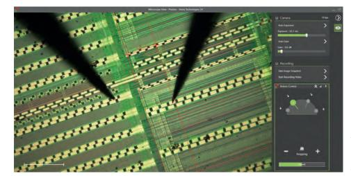
Precisio<sup>™</sup> software microscopewindow with controls for imaging parameters, tools for recording, annotation, and dimensional measuring.
