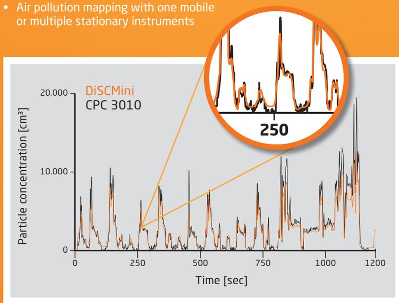
Compared to a small CPC DiSCmini is truly handheld, easier to use and also delivers an average particle diameter and lung-deposited surface area and not only the particle number concentration. DiSCmini measures size particles smaller than about half a micron correctly.
