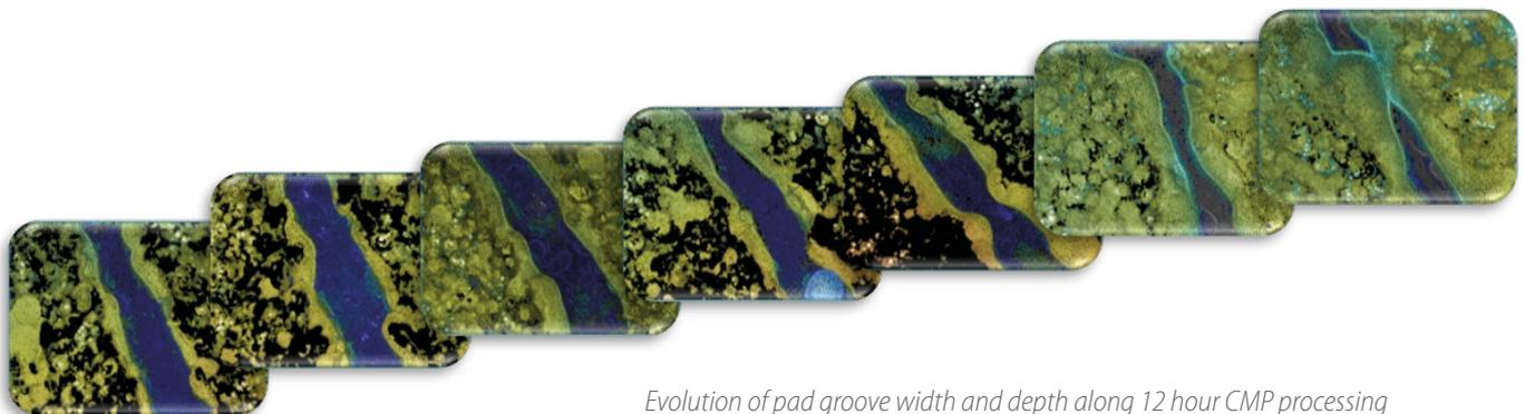
*Evolution of pad groove width and depth along 12 hour CMP processing*
